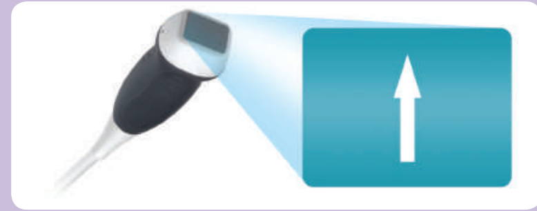
Single crystal material exhibits fewer poling variation
